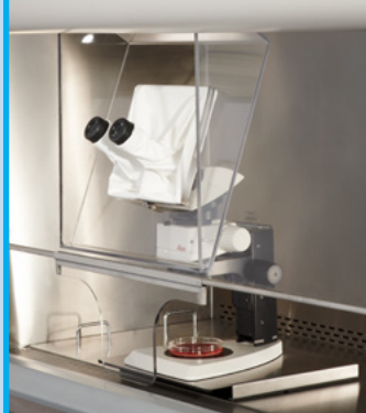
This LabGard® BSC was fitted with a microscope viewing window to accommodate workflow specializing in human cell tissue research.
