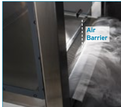
A dynamic air barrier at the front of the cabinet separates the laboratory from the work zone environment at an air speed of 105 fpm (0.53 m/s).
