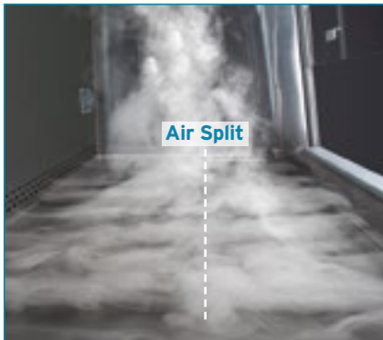
True laminar (unidirectional) downward moving air flushes the work surface at 60 fpm (0.30 m/s) minimizing cross contamination.
