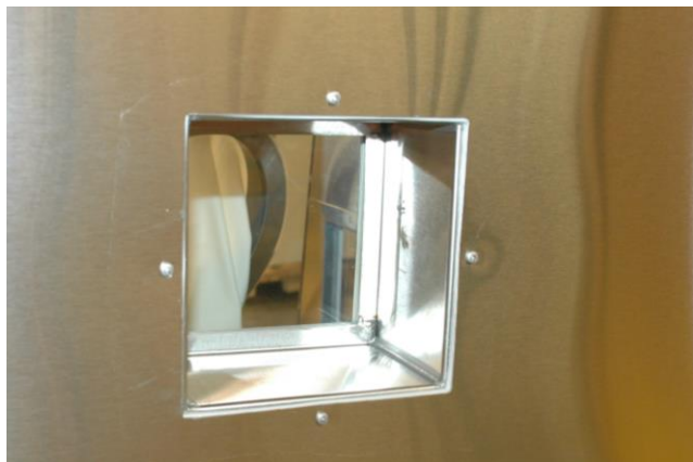
Photo 1 – View of camera and access from back. 1' x 1' opening reduced to 6" x 6" using tape.
