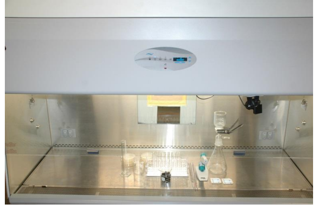
Photo 4 – View of Camera mounted on the control panel bottom right side to minimize operator interference.
