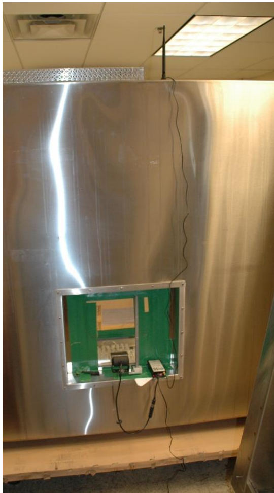
Photo 8 – Rear view showing RF transmitter and RF antenna
