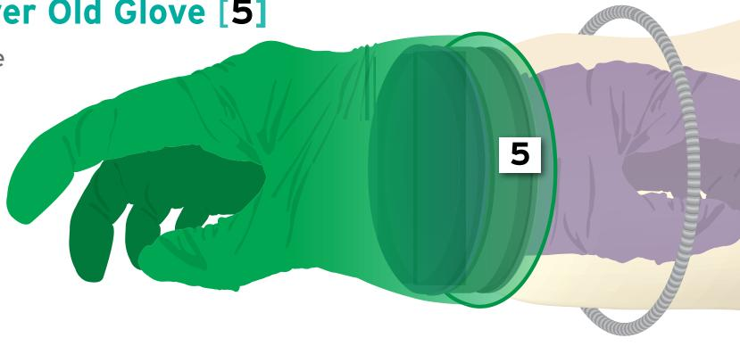
(F) Return Holding Spring to Second **Groove on Glove-Sleeve Ring [6]**
