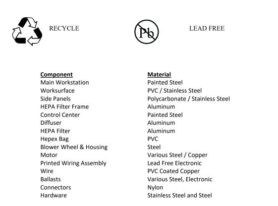
( Note: Material type can be verified with use of a magnet with stainless and aluminum being non-magnetic.
