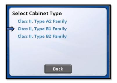
Note: If the BSC has a special downflow area (work zone), exhaust duct diameter size, or special work access opening window height, these must be entered into the control system to assure the correct display values. Press MENU to access these additional parameters. Select and SAVE appropriate size of each.
