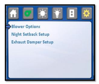
• Manual Blower control: When the manual blower control is on, the downflow and inflow displays will indicate nominal setpoints. Airflow adjustments can be made in manual mode by going into airflow calibration and adjusting the blower duty cycle. The blower duty cycle will remain constant in manual mode. The display will also indicate the manual control is activated. When the manual control is off, full automatic control resumes.
