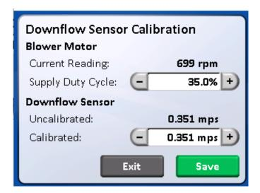
Step 5: Now, measure the average downflow velocity over the entire workzone using the recommended downflow velocity test grid (see Table 7.0).
