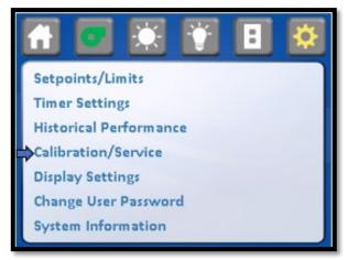
Entry into the Calibration/Service functions requires a service password for entry. After pressing the Calibration/Service menu item, a password screen will appear. The default password is "9876". Once the service password is entered; the Calibration/Service menu will appear.
