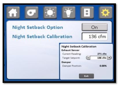
At this point, the night setback is active and the butterfly valve will begin to close. Now measure the inflow volume using a Direct Reading Instrument of inflow velocity measurement method. The goal is to reduce the inflow volume to a lower level that maintains a negative inflow velocity to save energy. This can be set at any other values within the damper operational range of 30% to 80%.
