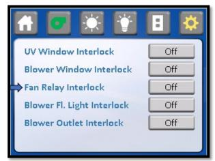
■ **Blower FL Light Interlock**: This parameter allows for the selection of the FL light option to be interlocked to the blower. When the blower FL light interlock is on, the FL light operation will be interlocked to the blower. When the blower FL light interlock is off, the FL light can be turned on at any time.
