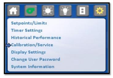
Entry into the Calibration/Service functions requires a service password for entry. After pressing the Calibration/Service menu item, a password screen will appear. The default password is "9876". Once the service password is entered, the Calibration/Service menu will appear. To exit, either press the menu or home icon.
