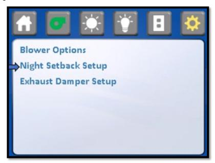
Step 1: Determine how night setback is initiated. If using contacts on main control board, proceed to step 2 Step 2: If using the display icon, enable night setback option by performing the following:
