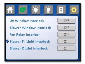
■ Blower Outlet Interlock: This parameter allows for the selection of the outlet to be interlocked with the blower. When the blower outlet interlock is on, the outlet operations will be interlocked to the blower. When the blower outlet interlock is off, the outlet can be turned on at any time.
