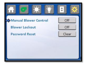
■ Blower Lockout: This parameter allows the access to turn the blower on or off to be restricted by the use of a password. When the blower lockout is on, pressing the blower icon will produce a numerical password screen. The default password is "1234" and may be changed using the password menu. When the blower lockout is off, the blower may be turned on and off without restriction.
