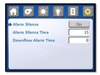
**Alarm Silence Time:** This parameter allows for the selection of time to determine how long the audible alarm shall be silenced. The time is displayed in minutes with a programmable range of 1 to 60.
