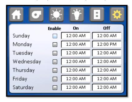
Once into the selected day, press on window to enter the on/off times. Use the keypad to enter hours or minutes. Press menu icon SAVE after each time entry. Repeat auto timer function for each day as desired
