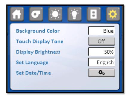
■ **Time/Date:** This menu item provides the ability to set the time and date displayed on the LCD screen. Time displayed is real time and will not automatically adjust for day light saving time.
