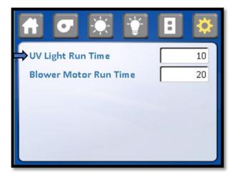
• UV Run time: This time shows how many hours the UV light has logged ON. Reset the time when replacing the V
