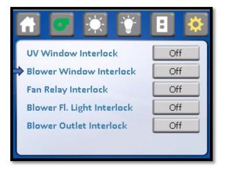
■ Fan Relay interlock: This parameter allows for the selection of the fan relay interlock operation. When the fans relay interlock is on, and the blower switch is pending or blue, the fan relay will be off or not energized. If the fan relay interlock is off and the blower switch is pending or blue, the fan relay will be on or energized. In either case the fan relay will be on when the blower switch is on or green and off when the blower switch is off or not colored.
