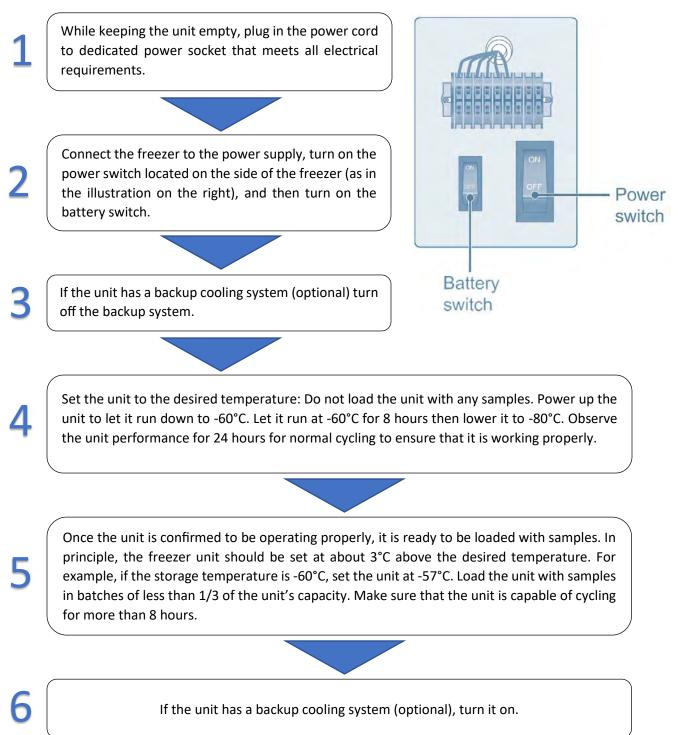
Your ULT unit should be cared for by trained personnel. Every 2 to 4 hours, the Unit's working status should be inspected and recorded daily. Should there be a malfunction in the unit, the freezer temperature rises. If the problems cannot be corrected in a short time, remove the stored samples, move them to another unit that meets the temperature requirements to avoid potential damage to samples.
