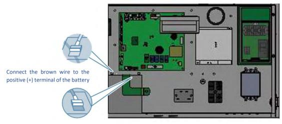
Connect the blue wire to the negative (-) terminal of the battery
