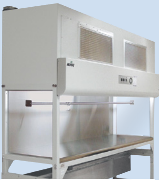
This Class I BSC was created at a nominal width of 8' [2.4 m], with clear polypropylene sidewalls, and a custom mounted IV bar.
