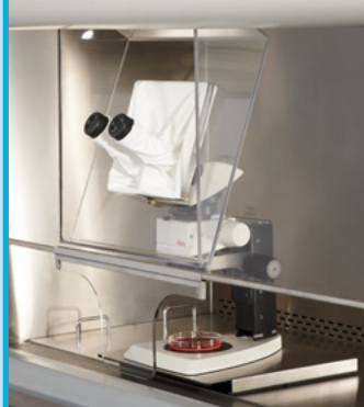
This LabGuard BSC was fitted with a microscope viewing window to accommodate workflow specializing in human cell tissue research.
