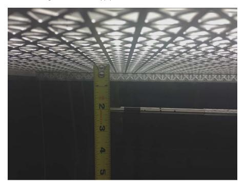
The exhaust flow is measured with a DIM (Direct Inflow Measuring) device placed over the exhaust opening and sealed off so that all the airflow into the exhaust chamber is flowing through the device.
