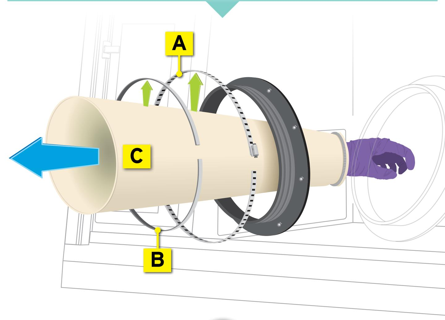
[D] Insert New Sleeve & Glove Assembly
