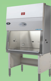
Type A2 70% Recirculated / 30 % Exhausted No Requirement to Externally Vent
