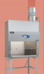
Type B1 30% Recirculated / 70% Exhausted Hard Connection External Vent
