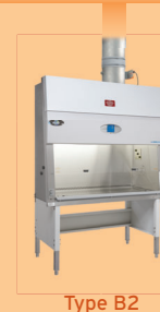
Type B2 0% Recirculated / 100% Exhaust Hard Connection External Vent
