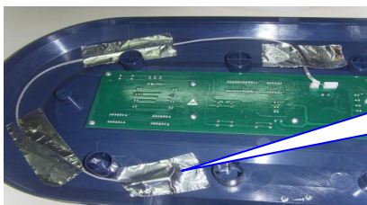
Ambient temperature sensor failure E0
