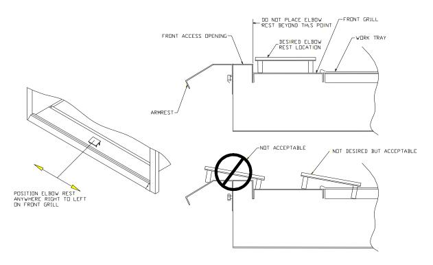
The BSC elbow rest is autoclavable or can be disinfected with a decontaminate, such as alcohol. **DO NOT USE CHLORINATED OR HALOGEN MATERIALS AS THEY MAY DAMAGE THE STAINLESS STEEL.**
