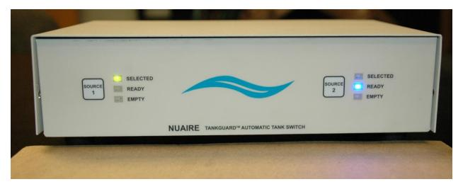
If for some reason, the original gas tank was not replaced and the secondary source gas tank was empty, the second internal pressure switch will detect the low pressure and change back to the original source. Again, during the automatic change, an audible alarm will sound and not having pressure on the original tank, will cause the audible alarm to stay on and only can be silenced by turning off the main power switch.
