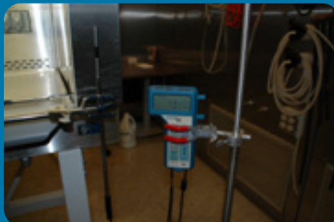
Thermal anemometer reading of 73 fpm within 2 inches.
