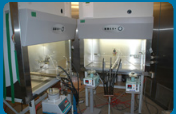
Personnel protection test of adjacent BSC's
