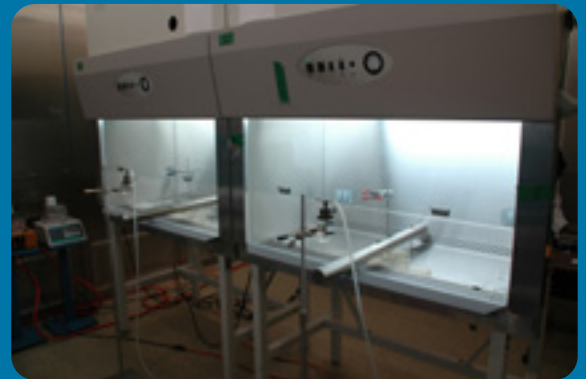
Product protection test of side by side BSC's
