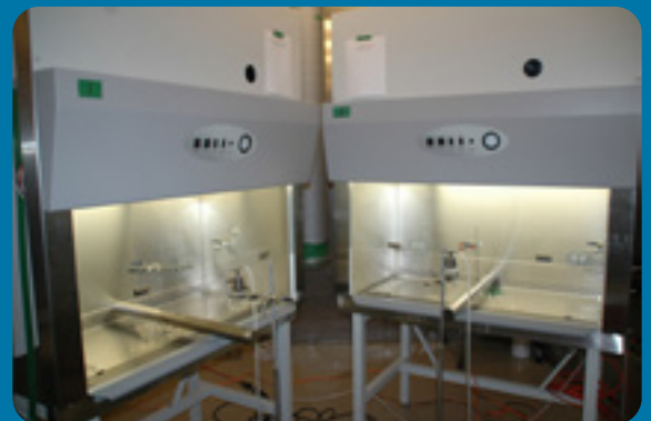
Product protection test of adjacent BSC's
