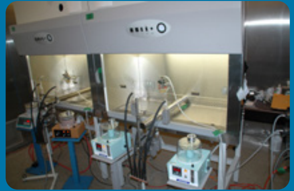
Personnel protection test of side by side BSC's
