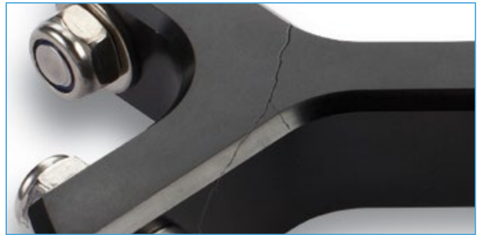
Crack in a Centrifuge Rotor
