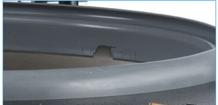
Damage to Lid Gasket
