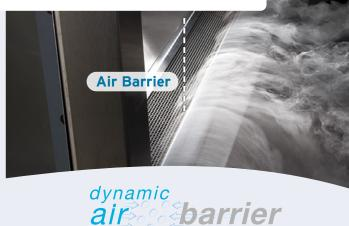
Class II BSCs create a dynamic air barrier at the front of the cabinet, which separates the laboratory from the work zone environment at a constant air speed of 105 fpm (0.53 m/s).
