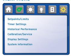
**Setpoints/Limits** - This controls the inflow & downflow air speeds and their allowable variance before sounding the visual/audible alarm.
