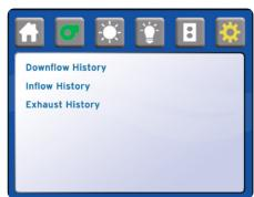
**Downflow History** - Displays downflow air speed setpoint and measured history from the last 7 days in the form of a line graph.
