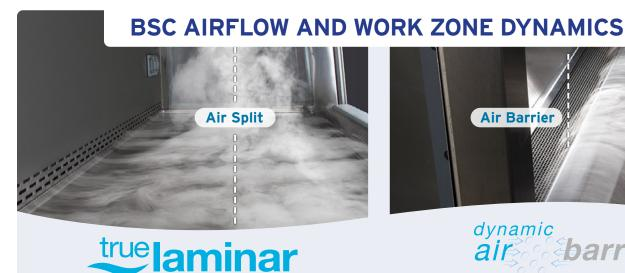
True laminar (unidirectional) downward moving air, utilized in class II biosafety cabinets, flushes the work surface at 60 fpm (0.30 m/s) minimizing cross-contamination within the work zone.
