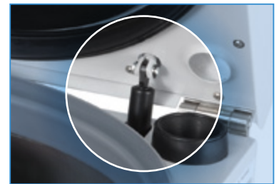
Centrifuge Lid Spring Mechanism, a potential point of failure.
