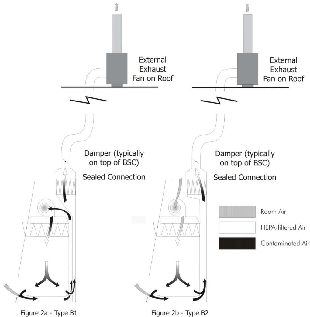
Figure 3 - Typical Type B exhaust systems
