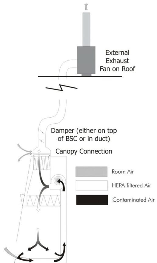
Figure 2 - Typical Type A exhaust system
